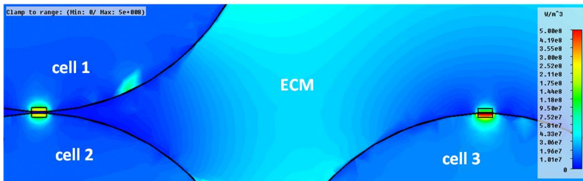
Figure 5. The particular nano effects in the cell membrane calculated by Computer Simulation Technology (CST) [4]. The point at touching two cells has concentrated energy absorption
