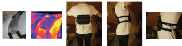
The electrode heats up the tissue but itself remains cold after 60 min treatment
