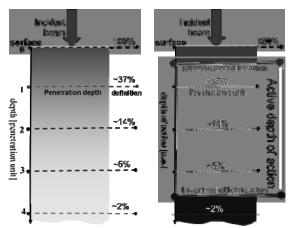
*Figure 3. The penetration depth is the distance where the initial beam energy (or field) decreases by ~63% (a). The real penetration from the point of view of the studied action is different (b).*
