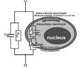
Figure 2. Electric schematics of one electrolyte "capsule", namely the cell.
