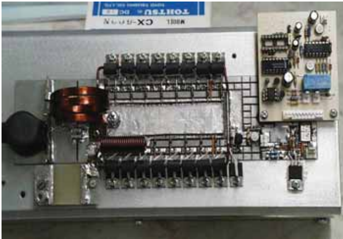
The first OncoTherm-made, “tandem” solid-state RF amplifier. (1993)
