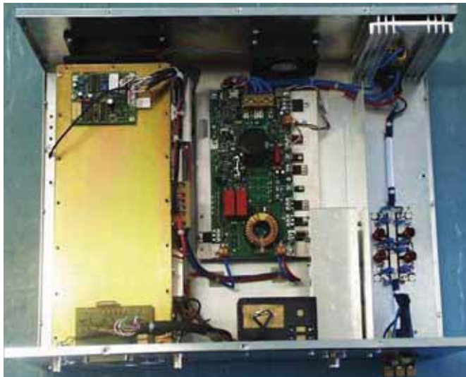
The high-level OncoTherm-made, new-principle E-class resonant solid-state RF amplifier. (2005) (The main unit of the amplifier is in the shielded box at left-hand side.)
