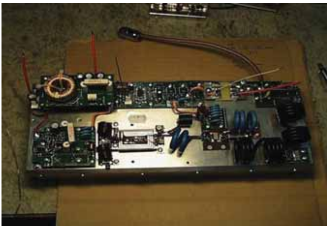
The first OncoTherm-made, E-class solid-state RF amplifier. (2003)
