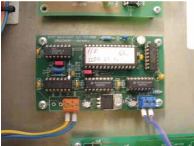
The modulation unit of the EHY systems
