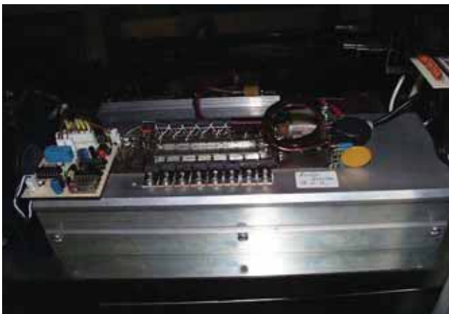
The first OncoTherm-made, linear (A-class) solid-state RF amplifier. (1998)
