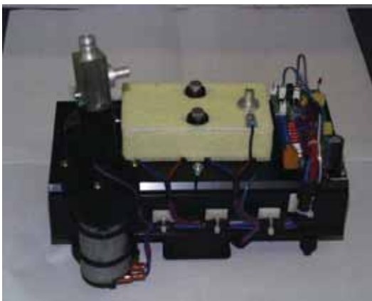
The cooling unit in EHY2000 systems
