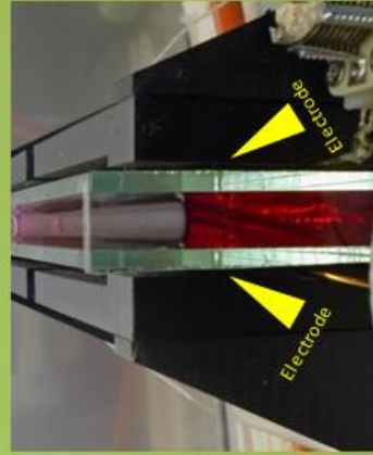
Lab-EHY 100 device electrode system for in vitro mEHT treatment
